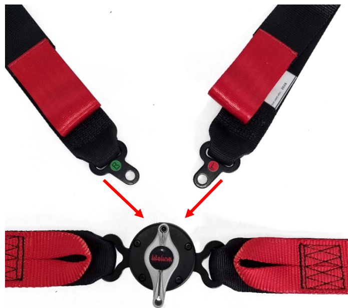
Figure 4: Shoulder straps instruction.
