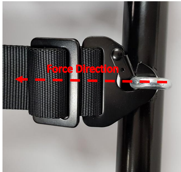
Figure 5: Force direction on snap hook.
